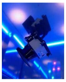
Once the owner get out from the entry cell, the system, through out some laser scanners, Will check the vehicle and his size, in order to verify they will be into the platform and avoid any car's damage, during the moving and parking process.
